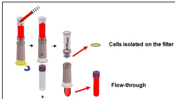
*Figure 1. Illustration of the ScreenCell® device operation. Diluted sample is placed in the sample reservoir. A vacuum is applied across the microporous membrane filter drawing fluid through the filter. The filter with captured cells is ejected from the device for further processing.*
